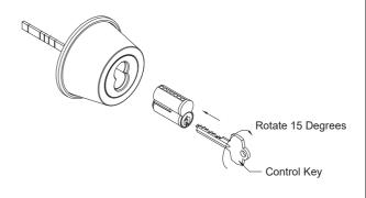
Caution: Double cylinder locks are operated by key only and may hinder emergency exit. Check for applicable fire codes and/or life safety codes before installing double cylinder gate latch bolt.
